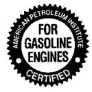
This symbol means that the oil has been certified by the American Petroleum Institute (API). We only recommend synthetic API Certified engine oils, such as Mobil 1<sup>®</sup>, that meet the requirements of Material Standard MS-10725. Use Mopar or an equivalent oil meeting the specification MS-
